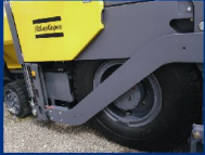
Techking 44/60R25 ETGC E2 Tire with Atlas Copco Paver
